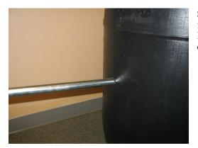
Step 6: Install aluminum tube (short) into one side of barrel as shown in fig. 5. Slide aluminum tube up to PVC tube assembly. Lift and rotate PVC tube assembly and slide same aluminum tube through next hole down. Continue sliding aluminum tube through opposite side of barrel.
